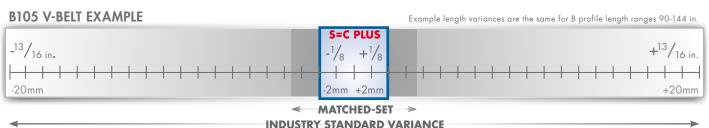
Industry standard length tolerances for a B105 v-belt will vary + or - 13/16" or more than 1-1/2". OPTIBELT Set-Constant (S=C PLUS) tolerances vary + or - 1/8" or only 1/4" **regardless of the date manufactured**.
